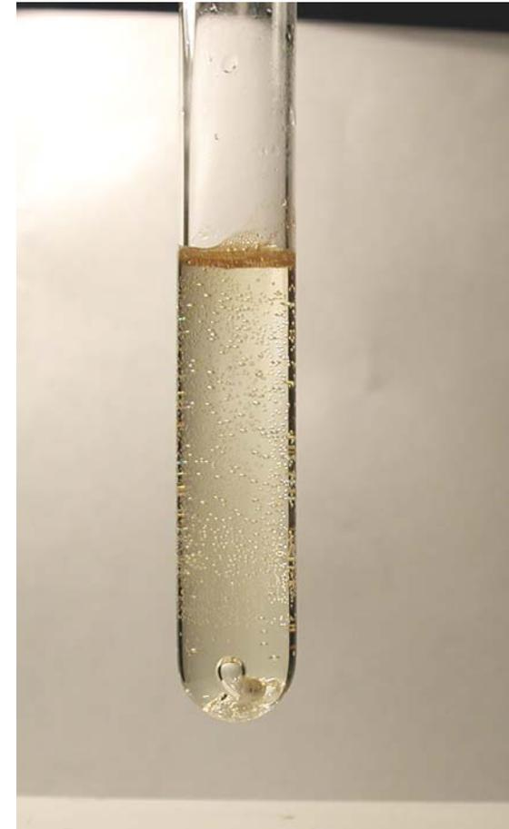
H<sub>2</sub> gas bubble evolution from the heavy metal halide reaction.
